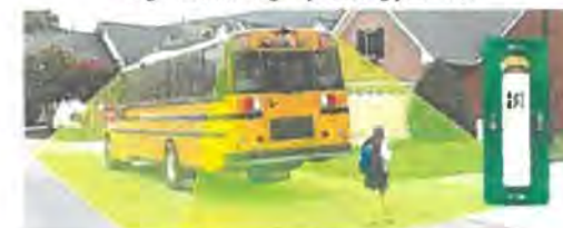
The PV360 multi-camera provides a 360° view of virtually everything surrounding the C2.
